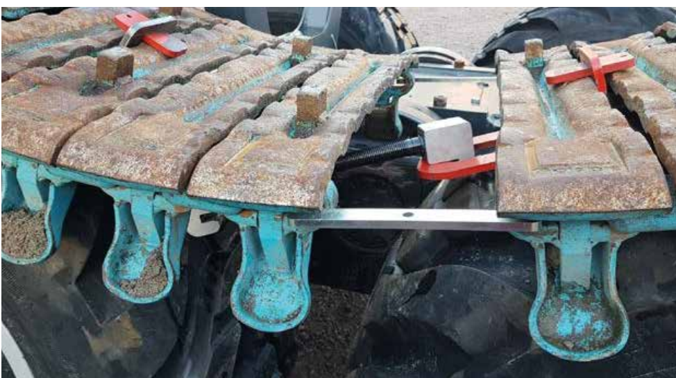
7a. Put tensioner hook to first pulling plate.
