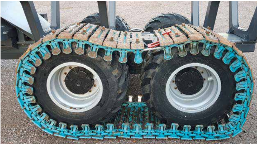
5. Place first pulling plate according picture and add securing plate.
