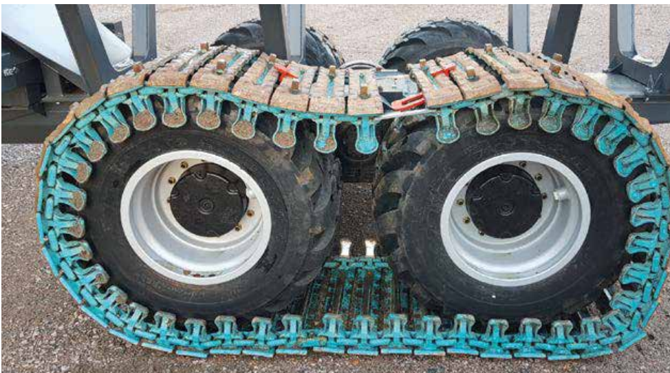
6. Place second pulling plate and add securing plate.
